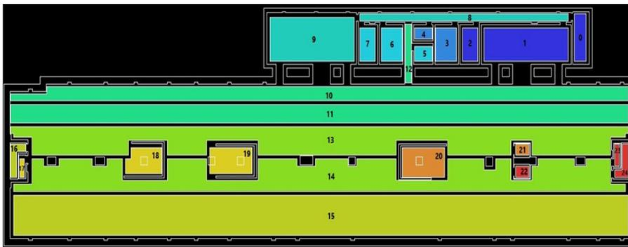
**Fig. 7. Convex Space Analyses using Space Syntax Method for Orientation on the Second Underground Floor at the Sa'at Square Station**
