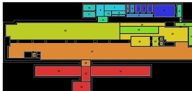
**Fig. 5. Convex Space Analyses using Space Syntax Method for Orientation on the Ground Floor at the Sa'at Square Station**
