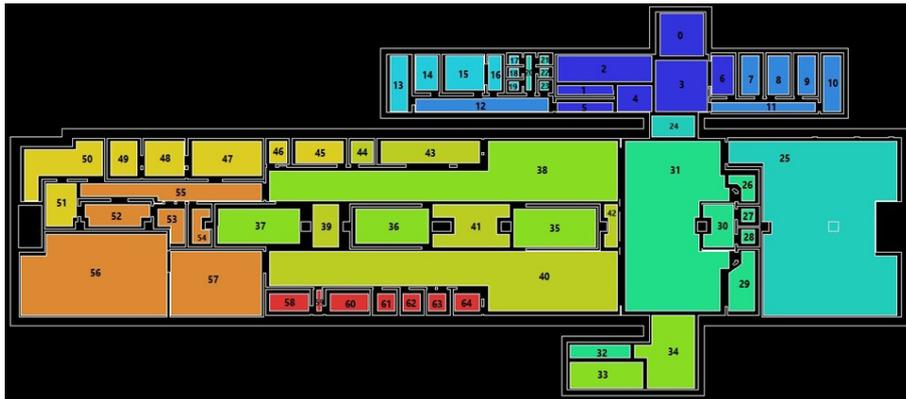
**Fig. 6. Convex Space Analyses using Space Syntax Method for Orientation on the First Underground Floor at the Sa'at Square Station**
