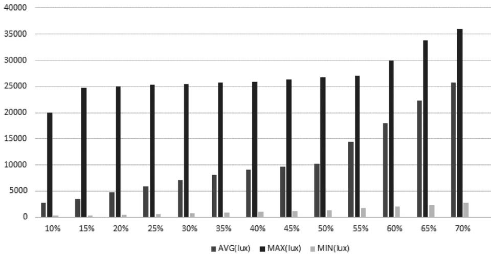
Fig. 7. Values of Illuminance (Light Level, in Lux) for Different Window Configurations
