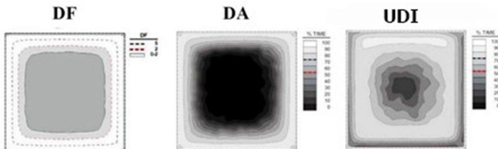
Fig. 1. Analysis of Daylight Conditions with Different Metrics in the AON Center Building by the Department of Building, University of Idaho
