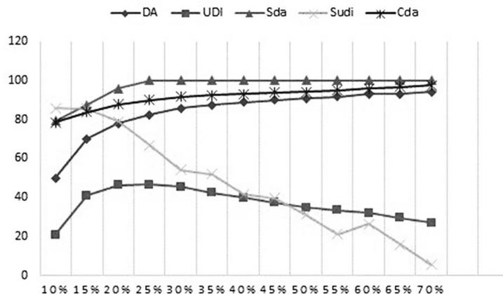
Fig. 9. Variation Trend of Dynamic Daylight Metric by WWR
