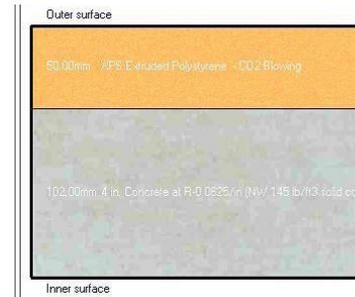
Fig. 10. Executive Specifications Solar Chimney Wall
