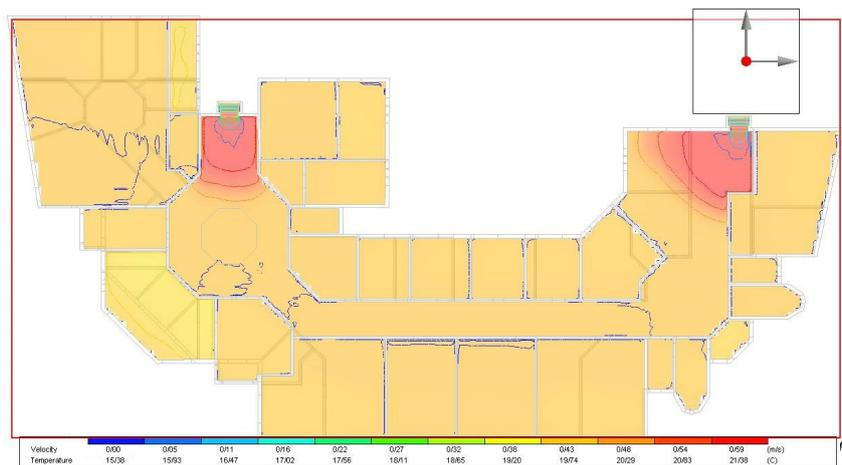
Fig. 11. Temperature Distribution in Building Floors after Applying Solar Chimney based on CFD
