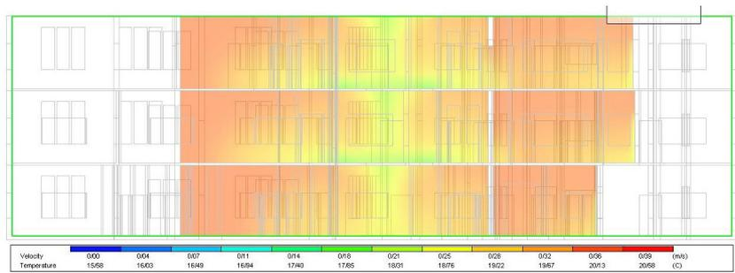
Fig. 7. Temperature Distribution in the Floor along the Chimney based on CFD
