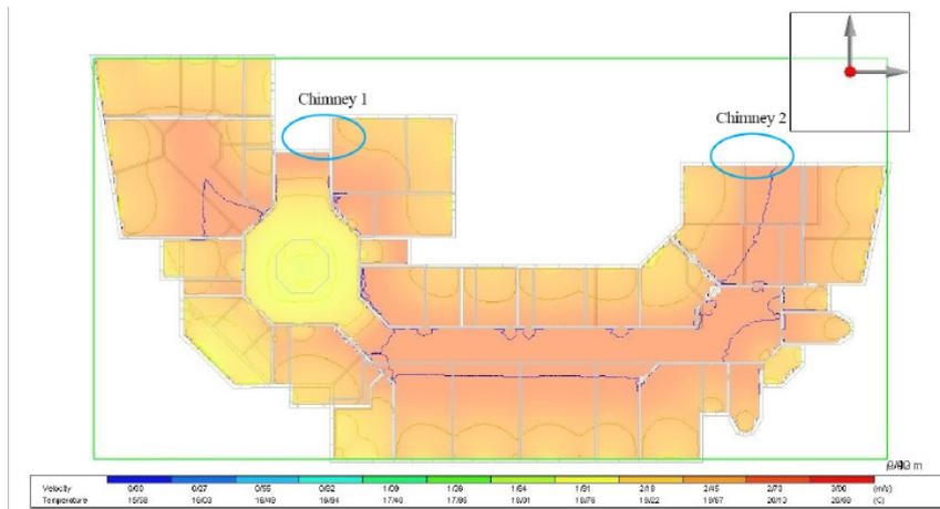
Fig. 6. Temperature Distribution on the Third Floor of the Building based on CFD
