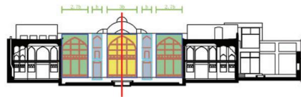
**Fig. 9. Symmetry in Parts and in whole on the Northern Façade of the Kadkhodaei House**
