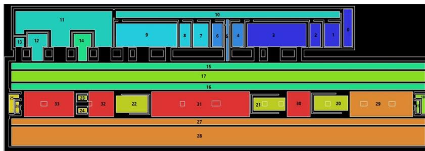
**Fig. 10. Convex Space Analyses using Space Syntax Method for Orientation on the Second Underground Floor at the Kohan Square Station**
