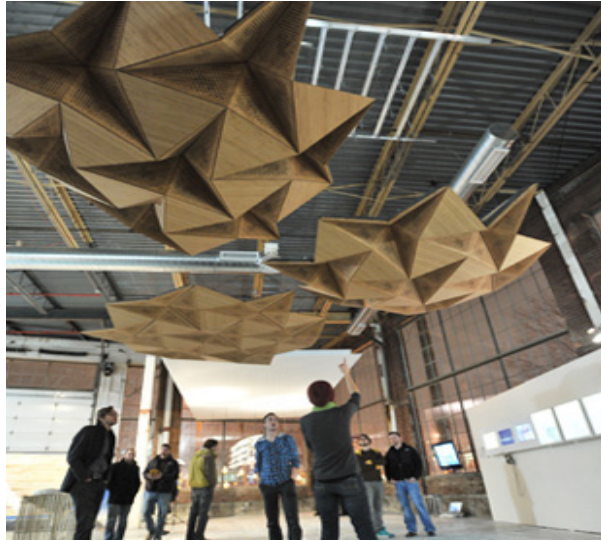
Fig. 3. Resonant Chamber, by RVTR Architects. These Acoustical Panels Expand and Contract Based on the Noise Conditions of the Adjacent Space, Picture Taken from (RVTR, 2011).
