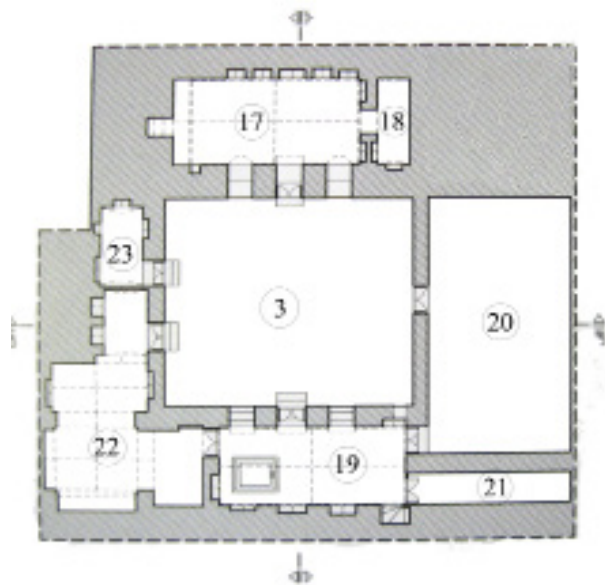
Fig. 13. Basement Floor Plan of Akhavizadegan Khaneh-Hussainia (Mohamadzadeh et al., 2007)
