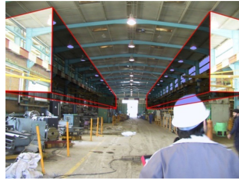
Fig. 3. Central Workshop of Tehran Refinery. Dead Spaces with No Use are Highlighted. All MVS is Off and the Gates are Open Instead.
