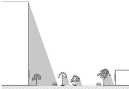
Fig. 8. The Position of Sun and Shadow in a Critical Spot of Nobahar Street, source; authors, 2019
