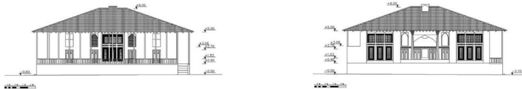
Fig. 10. Western and Eastern Facades of the Building
