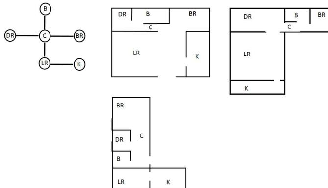
**Fig. 5. Different Plans with the Same Graph**
