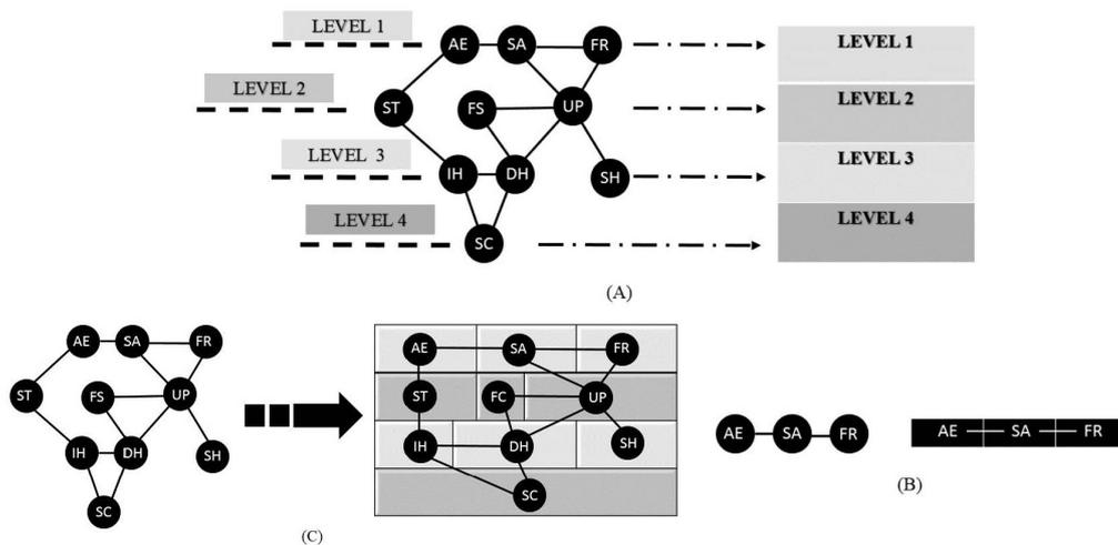
Fig. 3. A. Transformation of Neighborhood Graph Levels to a Rectangular Plan, B. Transformation of the First Row of a Graph to a Rectangular Plan, C. Transformation of the Neighborhood Graph to a Rectangular Plan (Liggett, 2000)
