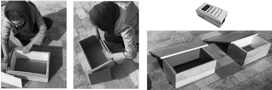
Fig. 6. Construction of Field Samples to Test Temperature Results by the Data Logger
