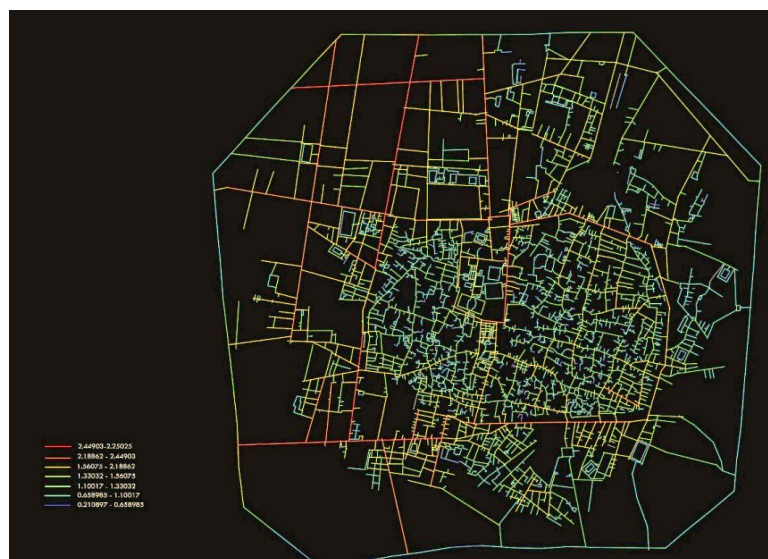
Fig. 6. The Axial Map used for Analyzing the Integrity Parameter using Depthmap Software; The Limits of Tehran City in the Qajar Period (Nasseri Wall), based on the Map drawn by Abdul Ghaffar
